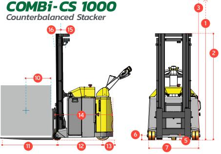
With a load capacity of 1000 kg @ 500mm the Combi-Counterbalanced Stacker (Combi-CS)can work in the smallest operating aisles.
